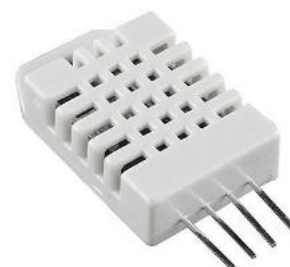
Figure 7: DHT22 Digital temperature and humidity sensor module AM230.
