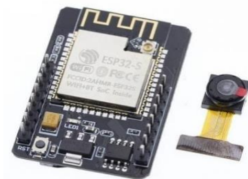
Figure 4: ESP32 CAM Wi-Fi module Bluetooth with OV2640 camera module 2MP.
