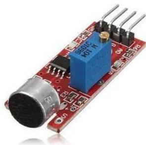
Figure 13: Sound detection module sensor for intelligent vehicle compatible with Arduino.
