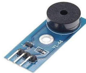
Figure 11: Active buzzer module 3.3V-5V.
