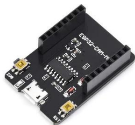
Figure 5: ESP32-CAM-MB MICRO USB download module for ESP32 CAM development board.
