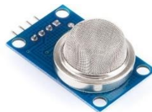
Figure 15: MQ-2 smoke LPG butane hydrogen gas sensor detector module.
